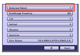
Adjust the level of Background Removal with "-" and "+", and then select "**OK**".
